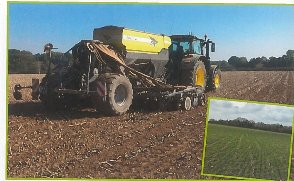
The JD6215R/Sky Easydrill combination direct drilling winter wheat after maize and (inset) the uniformity of germination and establishment.
